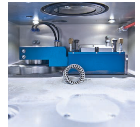
Schneller Prototypenbau durch Additive Fertigung Rapid prototyping by additive manufacturing
